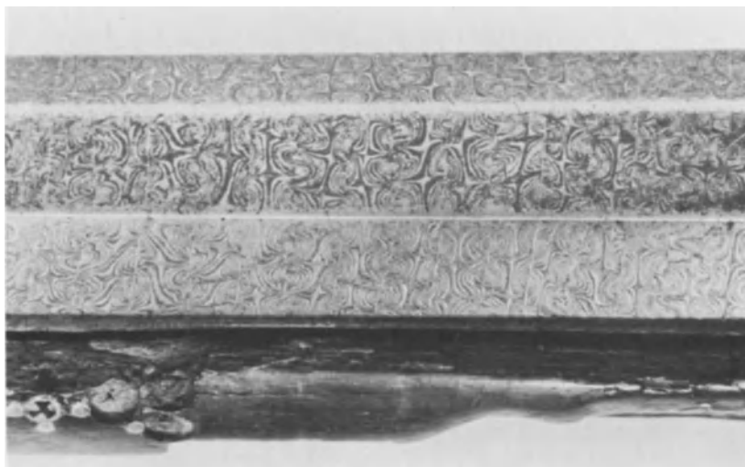
8. Turkish gun barrel of welded "Damascus" steel. XVIII cent. (Victoria & Albert Museum).
