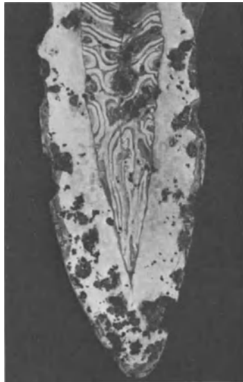
6. Merovingian pattern-welded sword, VI cent. A.D. Repolished and etched. 4.0 cm wide.
