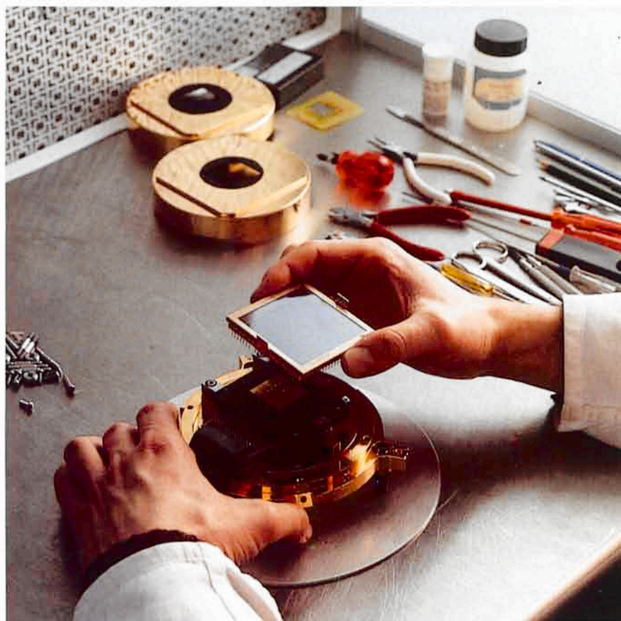
Figure 3: The first two 2048 2 pixel CCDs (the Ford Aerospace devices) have been successfully installed at La Silla in 1991. The coming addition to the ESO CCD family is shown in this photograph. It is a thinned, front-illuminated 2048 2 pixel Tektronix CCD with 24 \mu\text{m} pixel size. Shown is the engineering device which is used to test the electronics, the detector head and the dewar. Delivery of the scientific grade device is expected at the beginning of 1992. With its high quantum efficiency ( \text{QE} > 50\% from 450 to 850 nm) and low read-out noise the new CCD is expected to significantly enhance the performance of the EMMI spectrograph.
