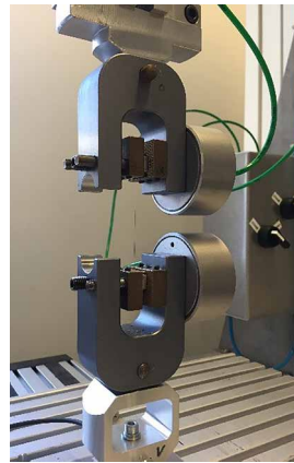
Fig. 1: Pull-Out tests of high-strength steel microfibers
