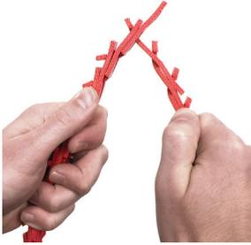
Holding belt with tabs to the outside push end tab through two links (three links for wedge profiles). Twist tab 90° into place.
