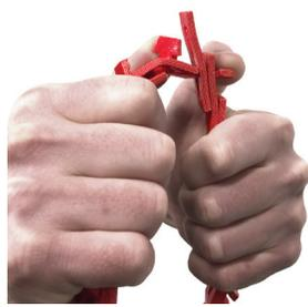
With your thumb twist second tab 90°. Push belt end down over tab with your opposite hand. For wedge profiles, repeat with remaining tab.
