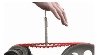
Using a force deflection gauge, check Installation force and confirm it meets the requirements below.
