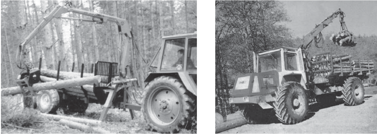
Fig. 7: Primary transport by a “ТП - 50Г(TP-50G)” cut-to-length trailer and “МСИ - 100(MSI-100)” forwarder
