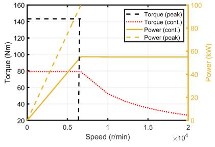
Target Torque Speed Profile
