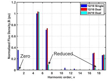
Normalized armature flux density in a 12 slot, 10 pole winding and a 24 slot, 10 pole space shifted dual three phase machine
