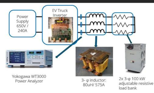
Inverter Test set-up at FREEDM
