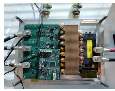
250kW, 800V SiC Inverter with > 98% efficiency
