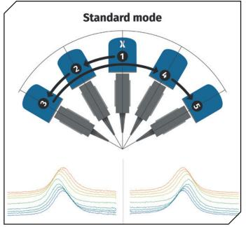
Figure 6 Standard mode x-ray diffraction systems use a timeconsuming sequence of individual scans.
