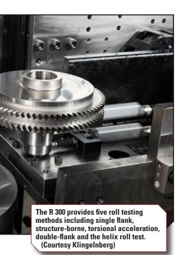
Looking into load-carrying capacity, the electric motor has a different torque characteristic increasing load on the drive flanks. In addition, recuperation leads to high loads on the coast side that is new to the automotive industry. Combining higher load and noise requirements in combination with a highly loaded coast flank, the optimization of a gear flank design becomes much more complex," Gorgels said.
