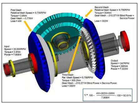
Figure 5 Energy loss per tooth mesh and efficiency calculation.
