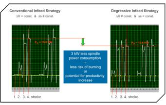
Figure 9 Graph demonstrates the spindle power comparison between infeed strategies.
