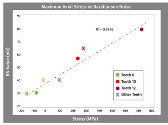
Figure 17 Data from MBN scans can be shown against simple rejection/acceptance criteria for easy evaluation.
