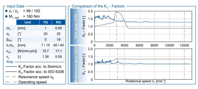
Figure 8 Comparison of the dynamic factors from SIMPACK and ISO 6336 (Ref. 27).
