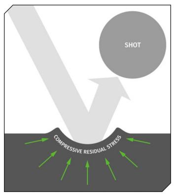
Figure 2 Shot peening results in a thin layer of compressive residual stress.
