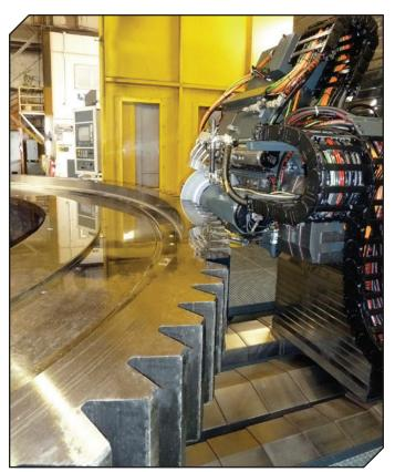
Figure 13 For large gears, the diameter of a grinding wheel is sized to reach the full depth of the gear tooth but also last long enough to avoid a mid-operation wheel change. Image Courtesy of Norton | Saint-Gobain Abrasives.
