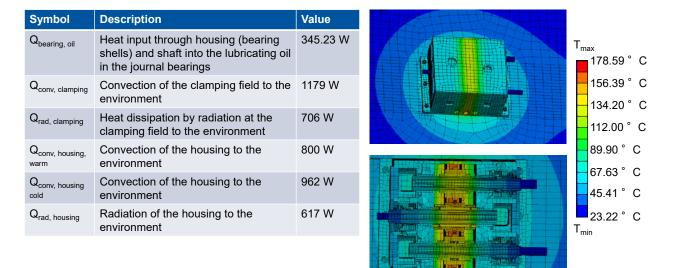
Figure 12 Results thermal simulation of the test gearbox with Ansys.
