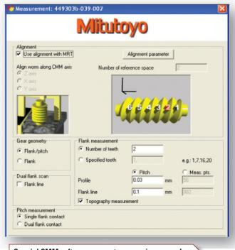
Special CMM software supports measuring several types of worm gears using a touch trigger probe or scanning probe on a CMM.
