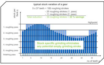
Figure 7 Stock-specific grinding eliminates the potential for empty grinding strokes.
