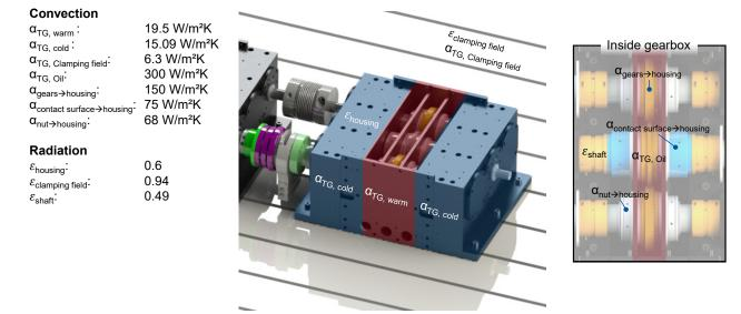
Figure 11 Overview of the boundary conditions of the test gearbox.
