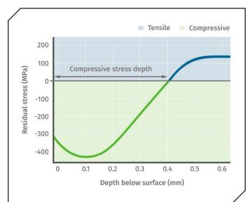
Figure 3 The compressive residual stress from shot peening can be a few hundred micrometers deep.
