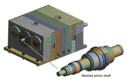
Figure 10 Meshed Ansys model of the test gearbox.
