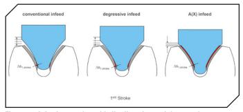
Figure 8 Infeed strategies with distributed material removal per stroke improves productivity and process reliability.
