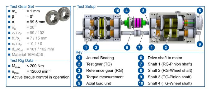
Figure 3 Design of the prototype test rig (Ref. 31).
