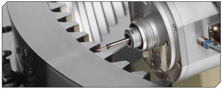
Figure 3 On-board inspection of both internal and external gears is fully integrated on Gleason machines.
