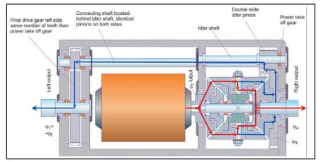
Figure 7 Double differential between the driving wheels—Solution 2.
