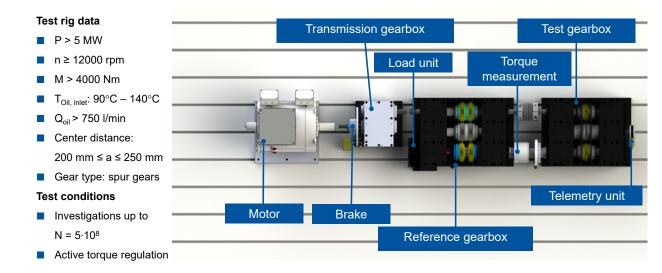
Figure 4 Design and power data of the main test rig for UHCF investigations under fully reversed bending.
