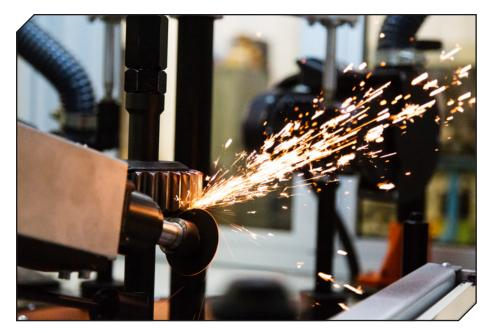
tangential positions, as well as tool speed, direction, and pressure. Crucially, this allows a single setup per part number, which can be consistently and reliably repeated simply by loading a program. With CNC ability, the TM 250 becomes a versatile workhorse for any gear manufacturers with a high mix of part types.
