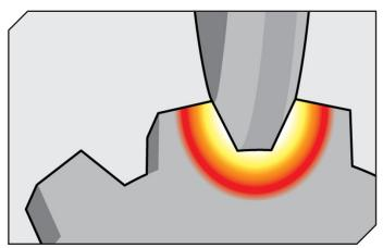
Figure 8 Aggressive feeds and speeds can result in grinding burn.
