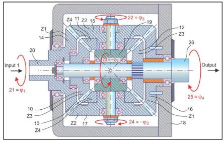
Figure 2 Double differential transmission.
