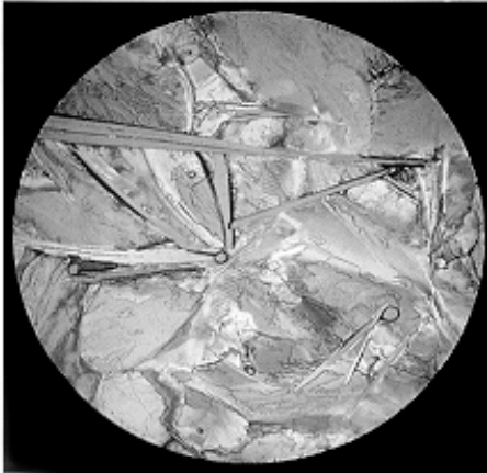
Fig. 5 40x magnification of a macrocrystalline stearic acid under polarized light.
