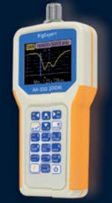
Antenna analyzer AA-230 ZOOM 0.1 - 230 MHz AS
