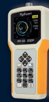
Antenna analyzer AA-55 ZOOM 0.06 - 55 MHz
