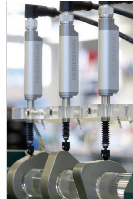
Testing station for flatness inspection
