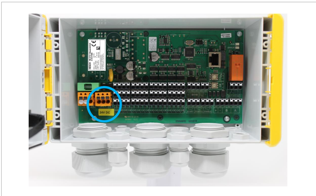
Figure 17. HE 5731 Compact with 24 V DC supply voltage (without connection adapter)
