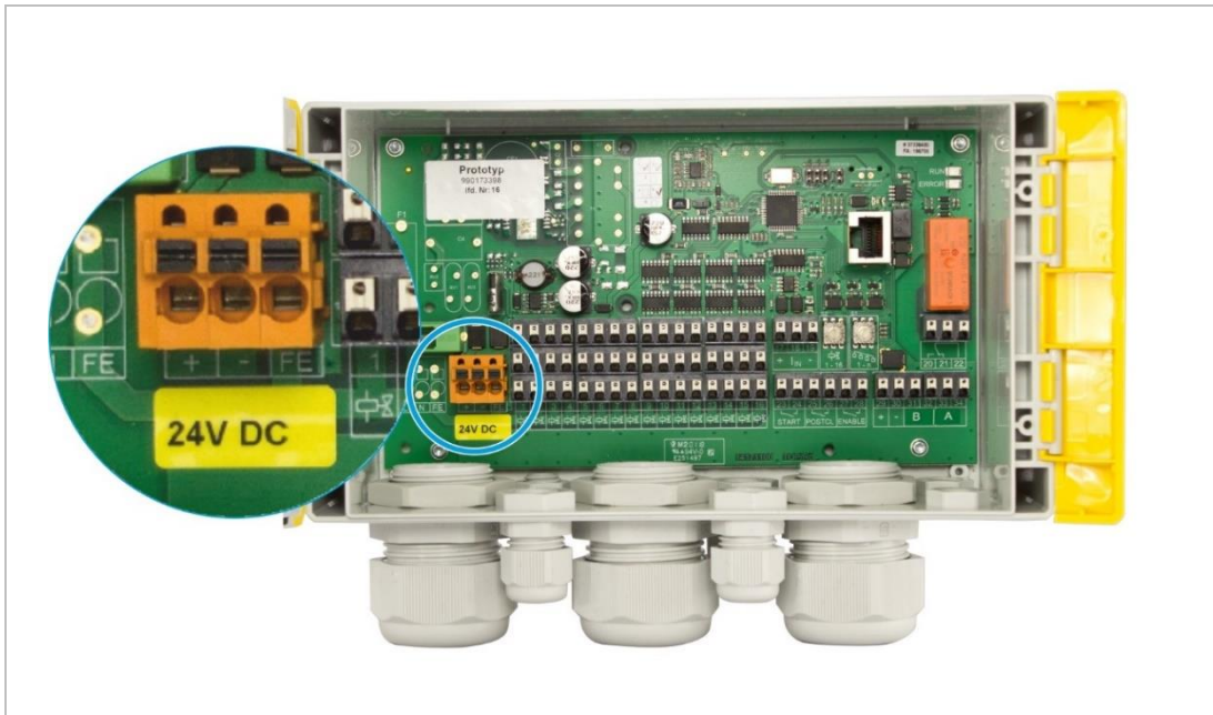
Figure 16. HE 5731 Compact with 24 V DC supply voltage (connection adapter optional)
