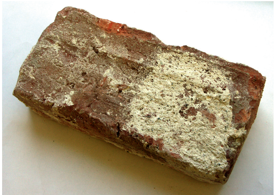
Fig. 2. Typical late medieval brick (22 × 10–10.5 × 5 cm) from Ebergassing Castle chapel, Lower Austria. Foto Paul Mitchell.
