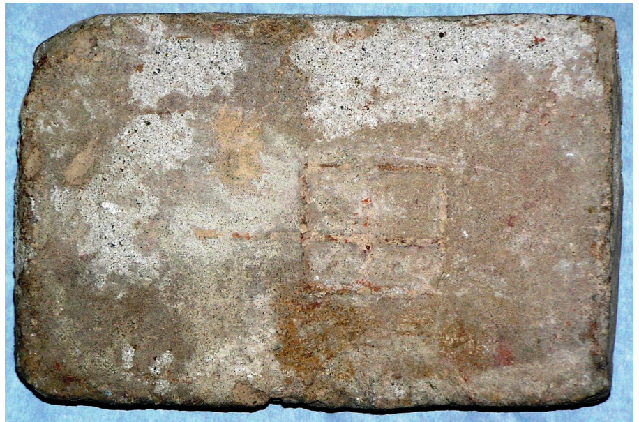
Fig. 4. Vaulting brick with raised grate mark (25–25.5×16×6–6.5 cm), St. Lawrence's Monastery brickworks, Vienna (1683–1783). Foto Paul Mitchell.
