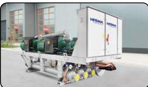
* Water-cooled chiller with inverter driven screw compressors installed in UK for chemical application. 600kW @ -2°C LWT
