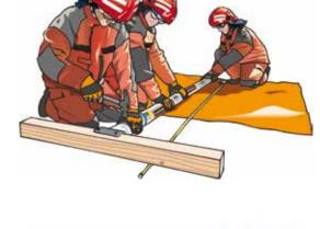
assemble your shore in a safe environment. A beam support head should be nailed to the center of the timber header.
