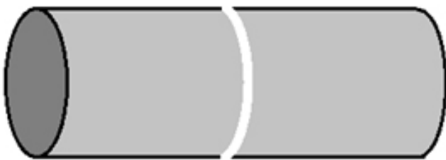
Figure 49 Cutting a pipe to make tags.
