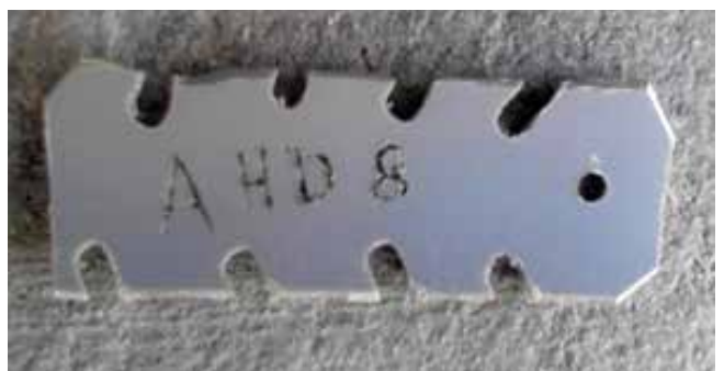
Figure 52 Above: Using a soldering iron to inscribe tags. Below: A finished tag.
