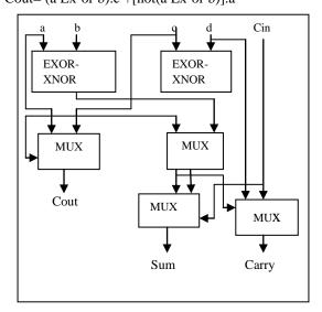
Fig.6: Logic diagram of 5:3 Compressor
