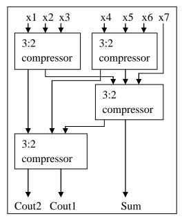
Fig.7: Logic diagram of 7:3 Compressor
