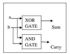
Fig.4: Logic diagram of Half adder
