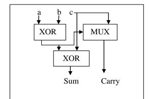
Fig.5: Logic diagram of 3:2 Compressor
