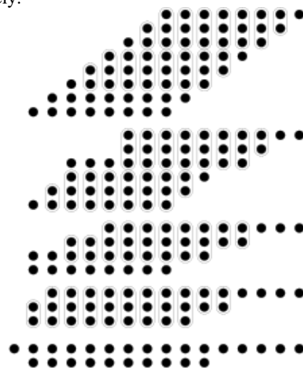
Figure 1: Dot structure for Wallace tree multiplier
