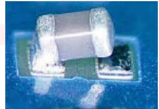
Fig. 1. With "tombstoning" only one side of a two-loaded chip component may be soldered to the target pad, but its other termination may not come in contact with the associated target pad. Photo courtesy of IPC-630
