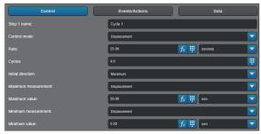
Making the test parameters user-driven variables gives you an easy way to rapidly change test parameters right from the operator screen. The powerful Bluehill® Universal Expression Builder makes this seamless in TestProfiler.
