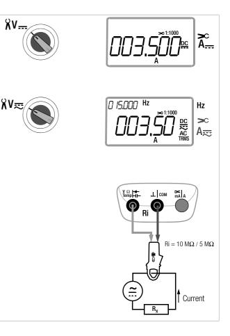
5.7.4 Alternating Current Measurement with Current Clamp Sensor, A AC and Hz  $\,$
