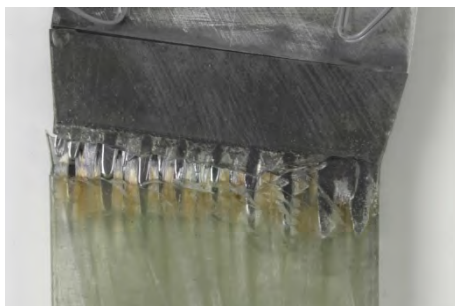
ALG8_BT2 ( F_{\max} = 54.3 kN)
