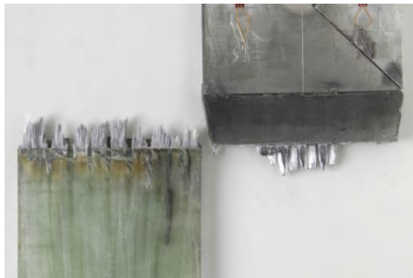
ALG8_BT1 ( F_{\max} = 67.7 kN)
