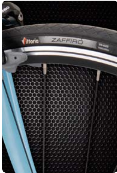
Vittoria Zaffiro 28c tires are just the right size for zipping through traffic: narrow enough to roll fast, wide enough to provide a secure contact patch. And there's plenty of frame clearance for even wider tires.
