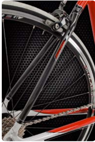
Adding a carbon fiber monostay to the Elite and Race enhances ride quality by damping road vibrations and optimizing lateral and torsional stiffness for out-of-the-saddle sprinting.
