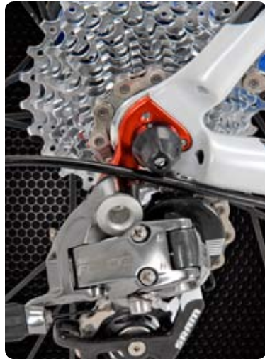
The Xenith dropouts are a solid, 1-piece forged design, as opposed to the standard 2-piece/bolt together type, reducing flex while enhancing structural integrity and frame longevity.
