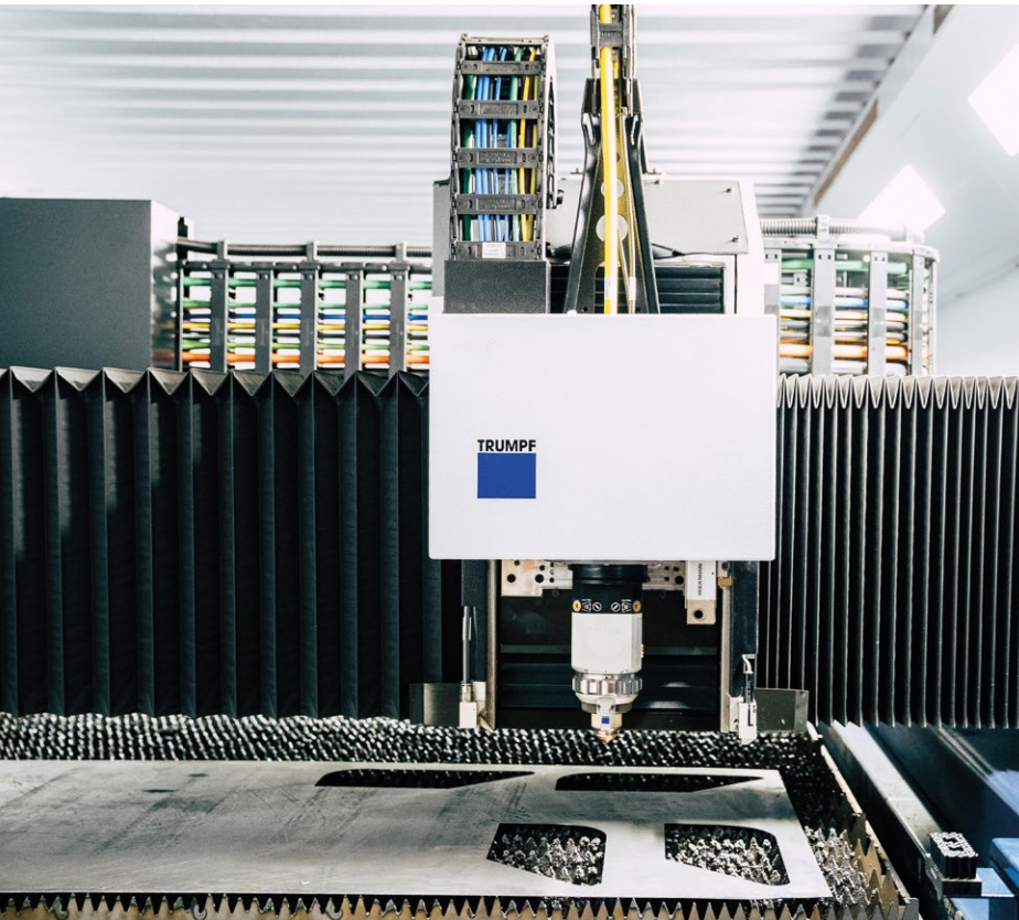
Trulaser 3040 Fibre laser with increased 4000 x 2000 bed size including integrated lift master and plate storage tower for unrivalled efficiency in parts production.
