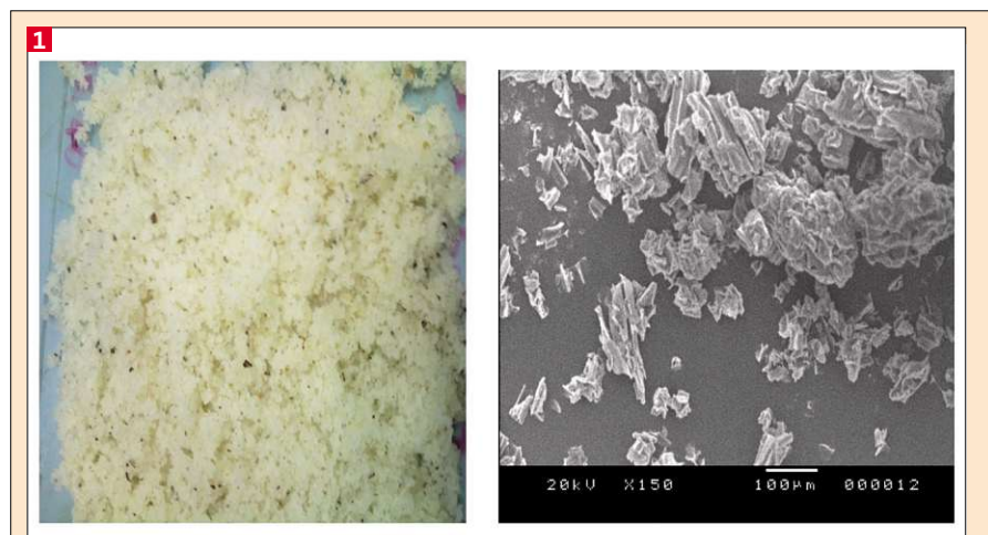
Fig. 1: Photograph image of CF filler and its morphology observed by SEM measurement
