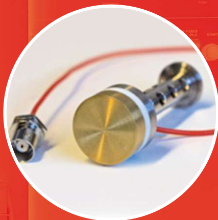
Exchangeable DEA/DMA-sample holder for compression mode
