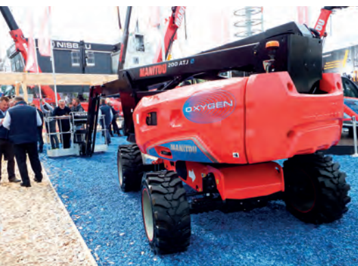
The ATJ 200 e, lead acid battery-powered boom from Manitou, shown at Bauma 2019.
