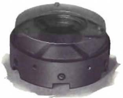
Right—Figure 17: Style KV thrust bearing for vertical shaft. Runner is shown in phantom. For vertical uses in its size range this is the most convenient form of six-shoe bearing, as it does not require a separate shoe-retaining flange. Style KBV (see Page 19) offers the same advantage in the larger sizes.
