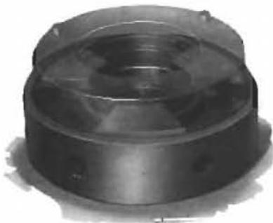
Left—Figure 16: Style LV thrust bearing for vertical shaft. Runner is shown in phantom. For vertical uses this is the most convenient form of three-shoe Kingsbury Thrust Bearing, as it does not require a separate shoe-retaining flange.
