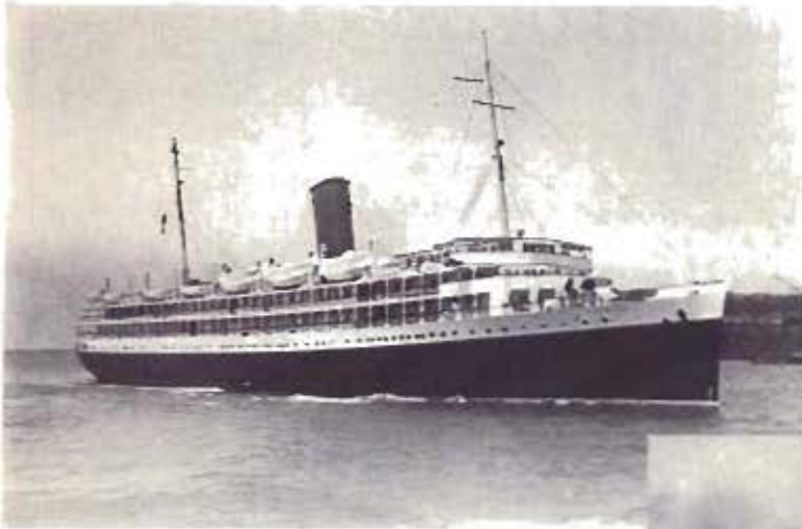
Above: S. S. "FLORIDA" of Peninsular and Occidental Steamship Company. 9,500 total shaft horsepower, twin-screw, geared turbine drive. Kingsbury Thrust Bearings used for propellers and turbines.
