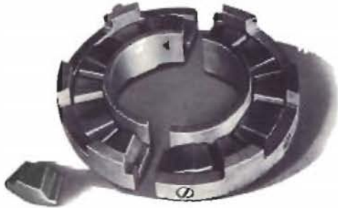
Figure 18: Style J bearing, with shoes removed to show leveling plates; also one separate leveling plate. Style J or B must be used where split construction is necessary for assembling. In vertical bearings a shoe-retaining flange is required either as an integral part of the thrust deck (see Figure 14) or as a separate ring (see Figure 32).
