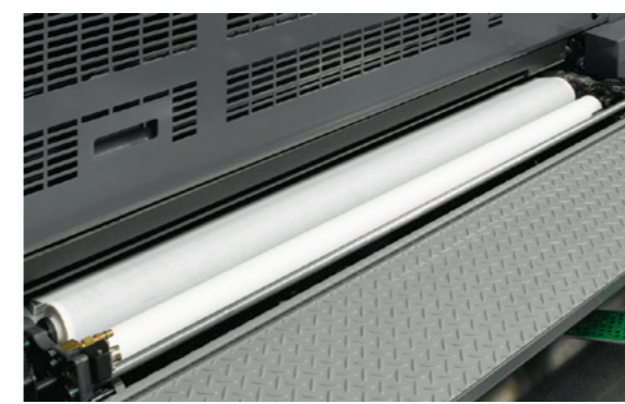
▼ Automatic Blanket Washer with Pre-soaked Cloth
