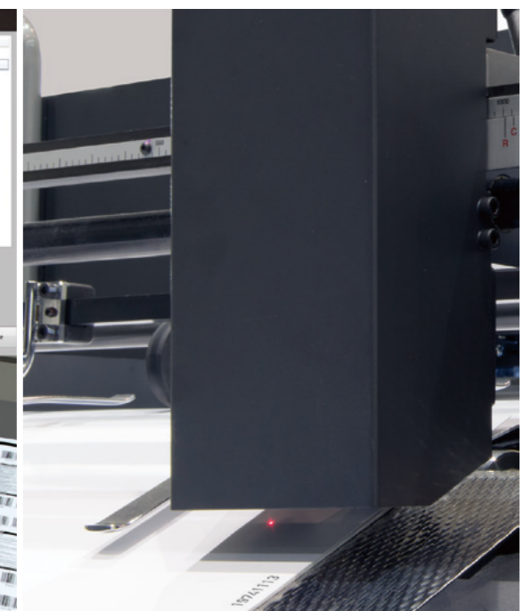
Sheet Numbering System (PQA-S option)
