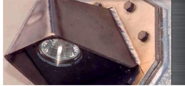
Titanium Light Assembly mounted to Steel deck with Titanium-Steel bimetal flange.
