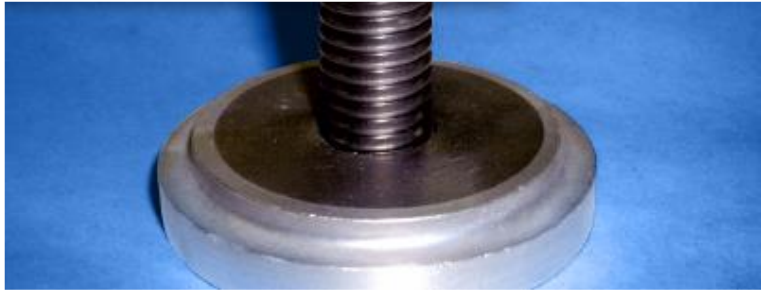
Titanium studs are welded to Aluminum hulls and decks
