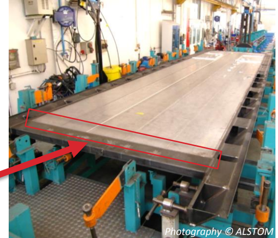
After: Aluminum alloy panel welded on the steel structure
