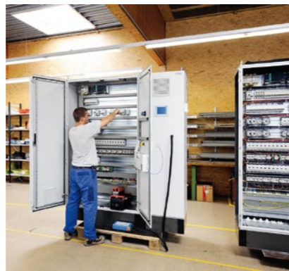
Control cabinet construction in the plant nearby
