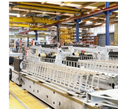
Assembly of the parts on the stacker crane mast
