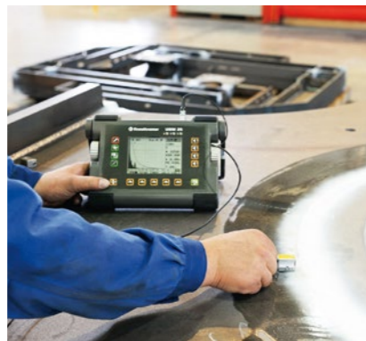
Ultrasonic testing of welded seams
