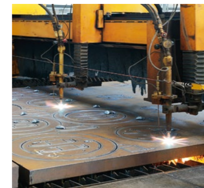
Oxyfuel cutting equipment
