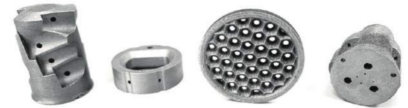
Components manufactured with Pacayal, a new austenitic stainless steel with a hardness of 40 HRC (Courtesy Kolibri Metals)
