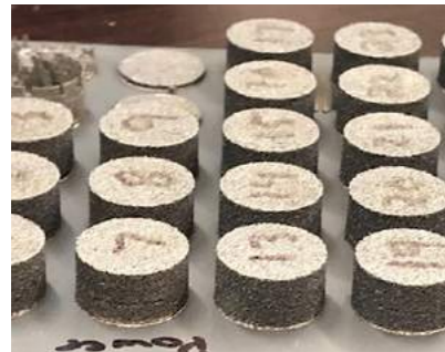
Additively manufactured test coupons of the ductile iron powder (Courtesy Mohawk College)
