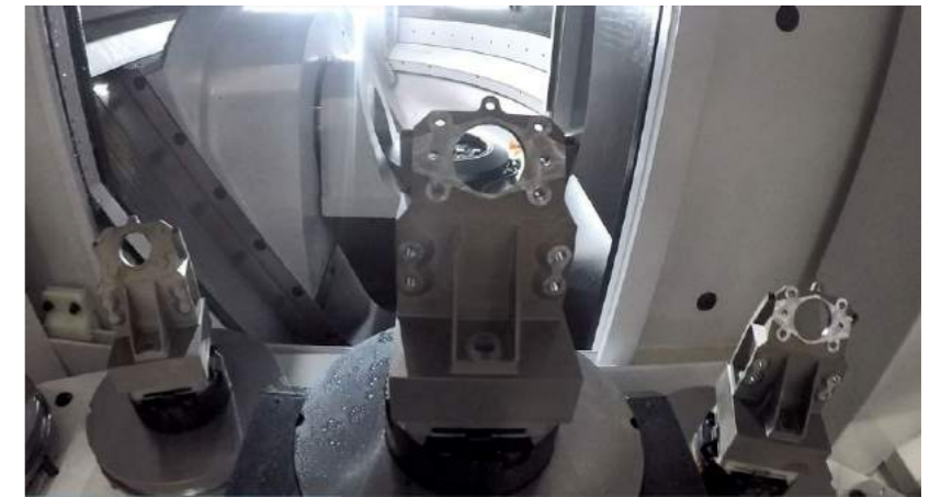
Fig. 6 BuildPal build plates benefit from the ability to use automated pallet handling for workflow optimisation (Courtesy System 3R)
