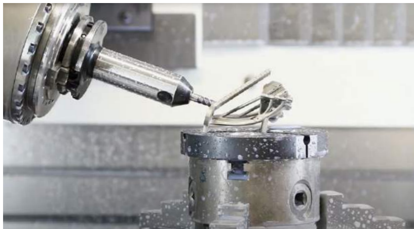
Bolt-It enables a post-process chain through automated gripping and handling of the AM part (Courtesy ETH Zürich, Inspire AG and Gressel)
