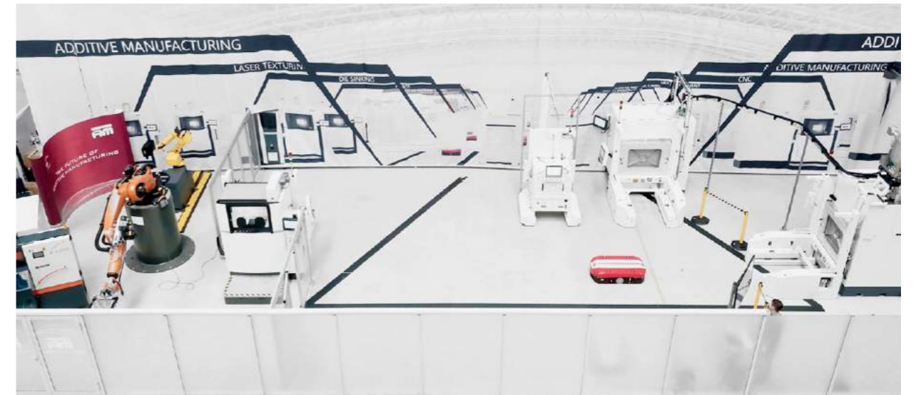
Fig. 5 As a collaboration between Premium AEROTEC, Daimler and EOS, NextGenAM was envisioned as a way to demonstrate the feasibility of an automated production cell for metal AM part production. A production unit was built at Premium AEROTEC's technology centre in Varel, Germany
