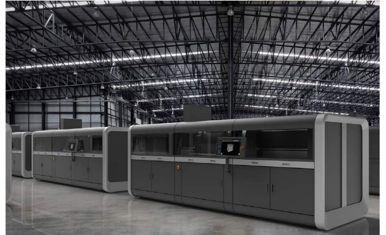
Fig. 3 The promise of high-capacity industrially focused metal Binder Jetting systems such as the Production system from Desktop Metal has served to highlight the potential of the process for mass production. However, the current reality of manually depowdering builds in such systems is a challenge that needs to be urgently addressed before Binder Jetting can be a true industrial-scale technology (Courtesy Desktop Metal)
