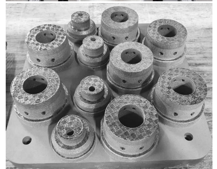
Fig. 4 Assembled multi-cavity injection moulding tool (top) and metal additively manufactured mould inserts (bottom) (Courtesy Berry Astrapak)
