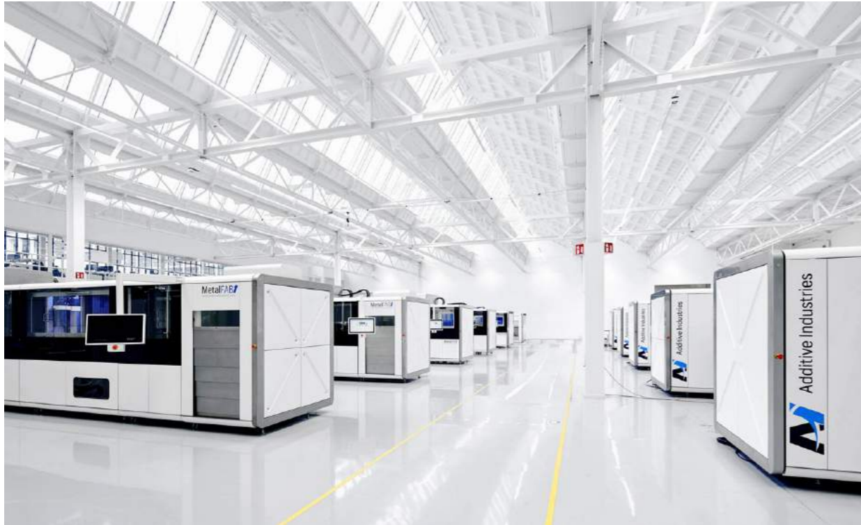
Fig. 8 The MetalFAB1 PBF-LB machine from Additive Industries has automation as part of its basic design concept, with connected modular units that include build 'cores', a powder removal unit, a heat treatment unit and a part removal module (Courtesy Additive Industries)
