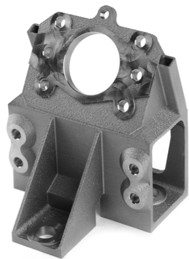
Fig. 5 An aerospace satellite bracket case study developed with 3D Systems utilising the System 3R system. Top: parts arranged on individual BuildPal build plates; middle: a part on a BuildPal before machining (left) and after (right); Bottom: the finished part removed from the build plate (Courtesy System 3R)
