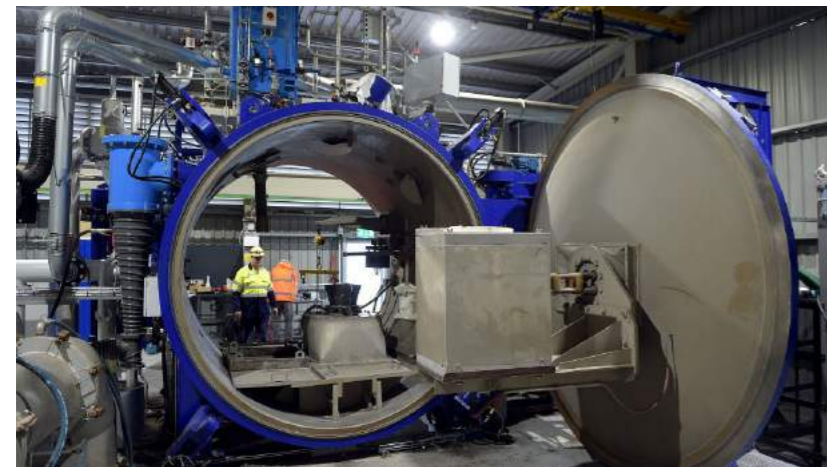
The atomiser at Liberty Powder Metals' new facility in Teesside, UK (Courtesy Liberty Powder Metals)
