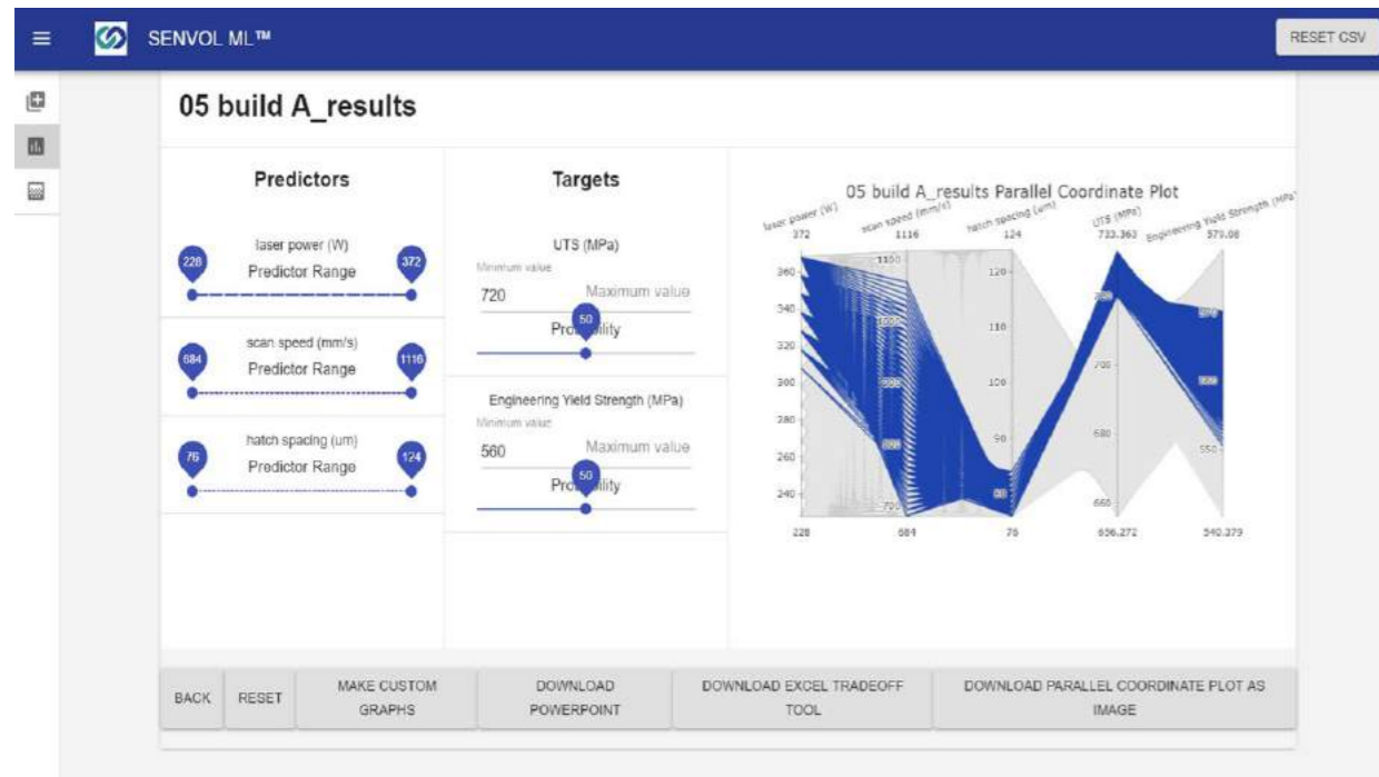
Fig. 4 Screenshot of the Senvol ML software interface. The parallel coordinate plot on the right shows the range of laser power, scan speed and hatch spacing an AM user should use if they would like to make stainless steel 316L coupons with 50% probability that UTS is 720 MPa or greater and 50% probability that yield strength is 560 MPa or greater
