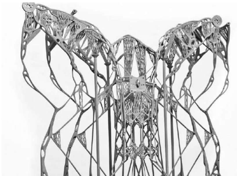
Fig. 9 Aeroswift machine (top) and drone body produced in its large build volume (bottom), measuring 542 x 542 x 141 mm [Courtesy ADC Aeroswift]
