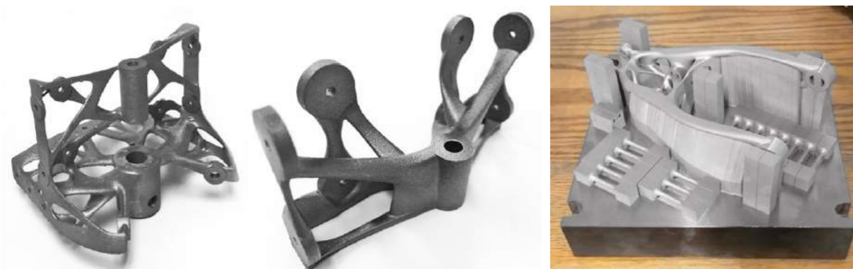
Fig. 3 Lower hinge bracket (left) and upper hinge bracket (centre) (Courtesy Aerosud). Nose wheel fork for AHRILAC aircraft (right) secured to build plate with support material intact (Courtesy Aerospace Development Corporation)
