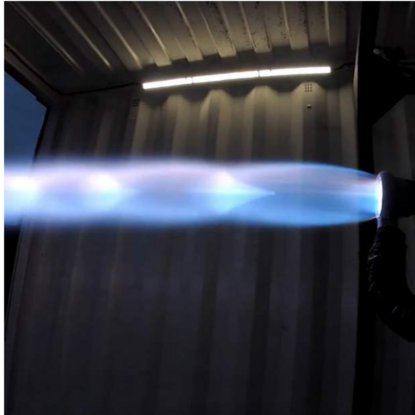
Fig. 6 Testing the E-1 engine. The blue mach or 'shock' diamond pattern in the supersonic exhaust plume is evidence of the efficiency achieved (Courtesy Launcher)
