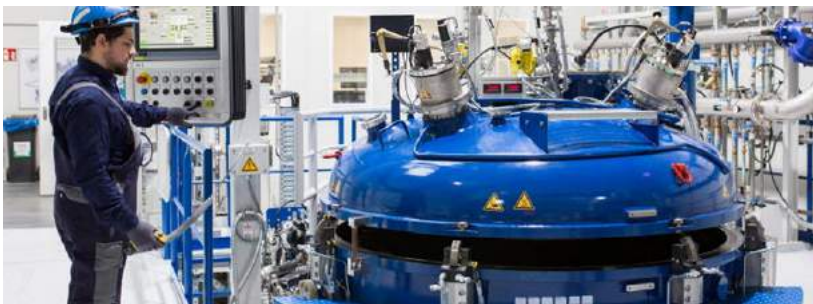
The new Vacuum Induction Gas Atomiser (VIGA) at its site in Laufenburg, Germany (Courtesy Höganäs AB)
