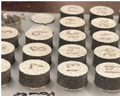
Additively manufactured test coupons of the ductile iron powder (Courtesy Mohawk College)
