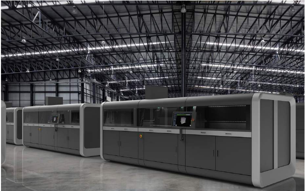
Fig. 3 The promise of high-capacity industrially focused metal Binder Jetting systems such as the Production system from Desktop Metal has served to highlight the potential of the process for mass production. However, the current reality of manually depowdering builds in such systems is a challenge that needs to be urgently addressed before Binder Jetting can be a true industrial-scale technology (Courtesy Desktop Metal)
