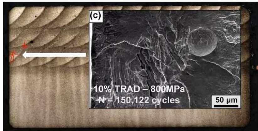
Dr Cameron Barr discussed macrostructure correlation in his presentation on the fatigue performance of steel repaired using DED (Courtesy RMIT University)
