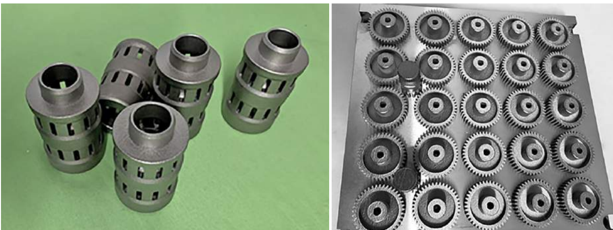
Fig. 6 Additively manufactured valve parts (left) and spares (right) (Courtesy Akhani 3D)
