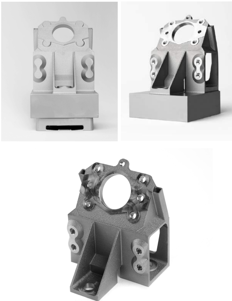
Fig. 5 An aerospace satellite bracket case study developed with 3D Systems utilising the System 3R system. Top: parts arranged on individual BuildPal build plates; middle: a part on a BuildPal before machining (left) and after (right); Bottom: the finished part removed from the build plate (Courtesy System 3R)
