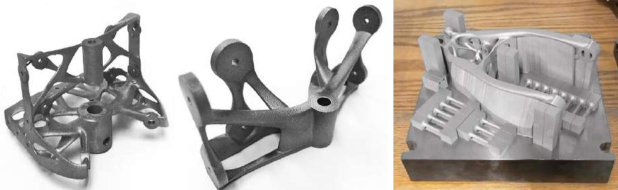
Fig. 3 Lower hinge bracket (left) and upper hinge bracket (centre) (Courtesy Aerosud). Nose wheel fork for AHRLAC aircraft (right) secured to build plate with support material intact (Courtesy Aerospace Development Corporation)
