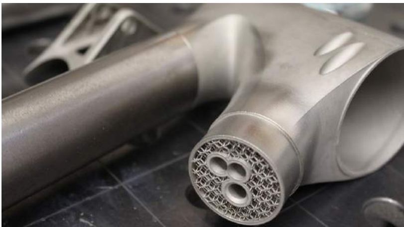
The Moorhuhn Bike combines titanium tubes with additively manufactured lugs (Courtesy Huhn Cycles)
