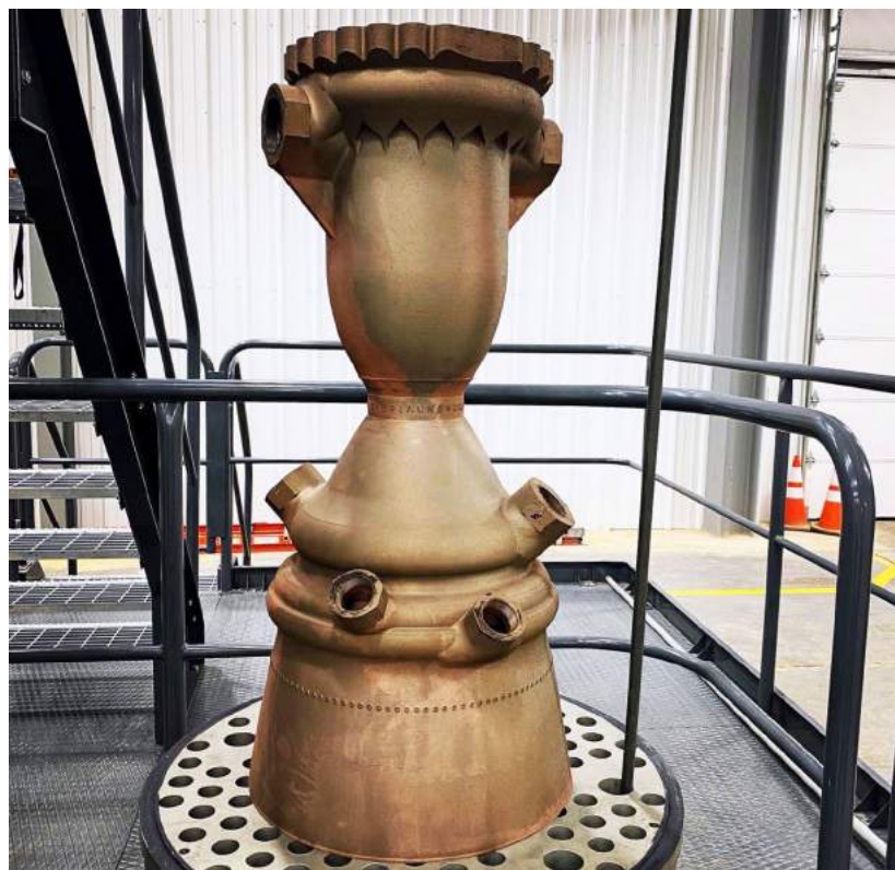
Fig. 7 The E-2 engine combustion chamber after heat treatment and Hot Isostatic Pressing (HIP) on a Quintus Technologies HIP system at Accurate Brazing Corp's Greenville, South Carolina, facility (Courtesy Launcher)
