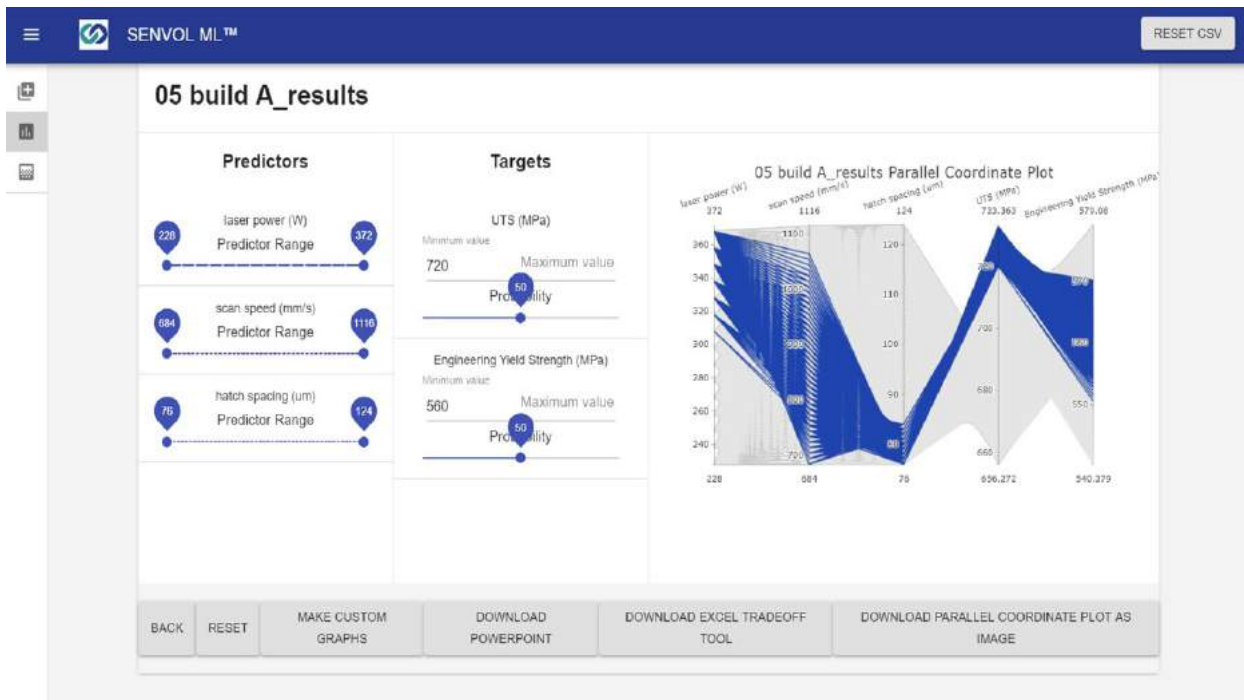
Fig. 4 Screenshot of the Senvol ML software interface. The parallel coordinate plot on the right shows the range of laser power, scan speed and hatch spacing an AM user should use if they would like to make stainless steel 316L coupons with 50% probability that UTS is 720 MPa or greater and 50% probability that yield strength is 560 MPa or greater
