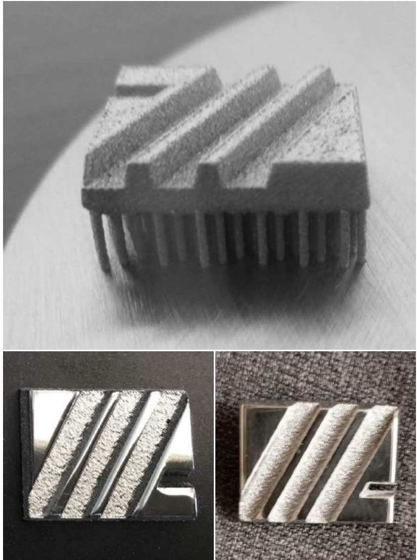
Fig. 7 Platinum Wohlers Associates lapel pin attached to build plate (top) and finished (bottom right). Titanium version (bottom left) (Courtesy Platform, Centre for Rapid Prototyping and Manufacturing)
