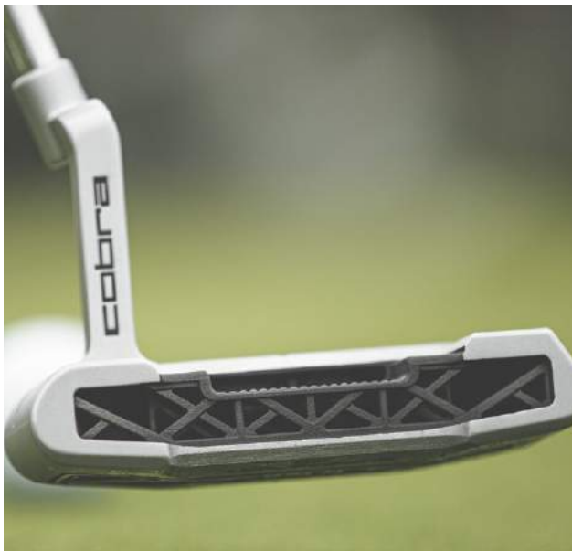
Fig. 1 The limited-edition putter features an additively manufactured 316 stainless steel body with an intricate lattice structure to optimise weight distribution (Courtesy Cobra Golf)
