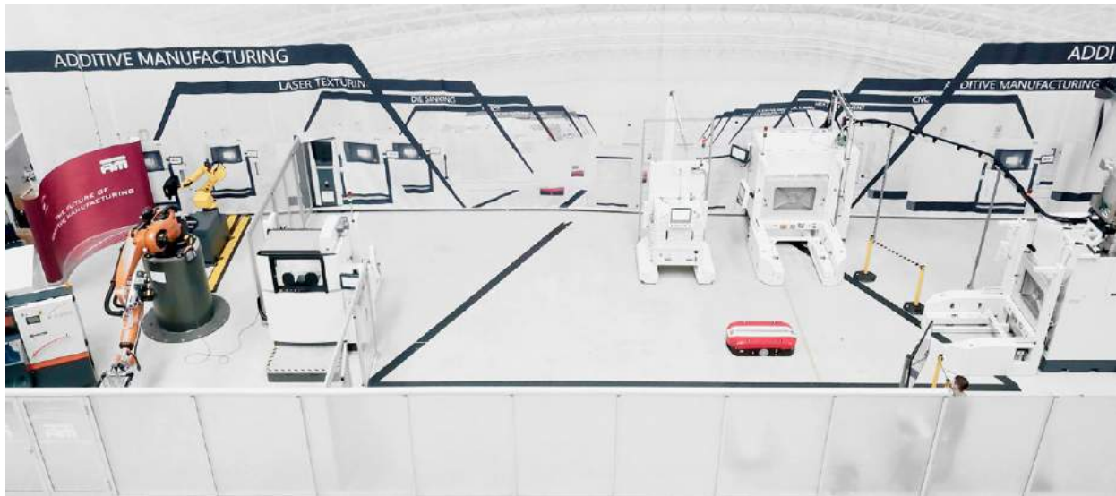
Fig. 5 As a collaboration between Premium AEROTEC, Daimler and EOS, NextGenAM was envisioned as a way to demonstrate the feasibility of an automated production cell for metal AM part production. A production unit was built at Premium AEROTEC's technology centre in Varel, Germany
