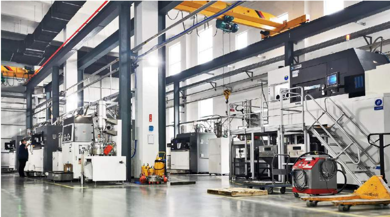
Fig. 2 Falcontech's Super AM Factory, which currently houses twenty-four Farsoon metal AM machines (Courtesy Falcontech)
