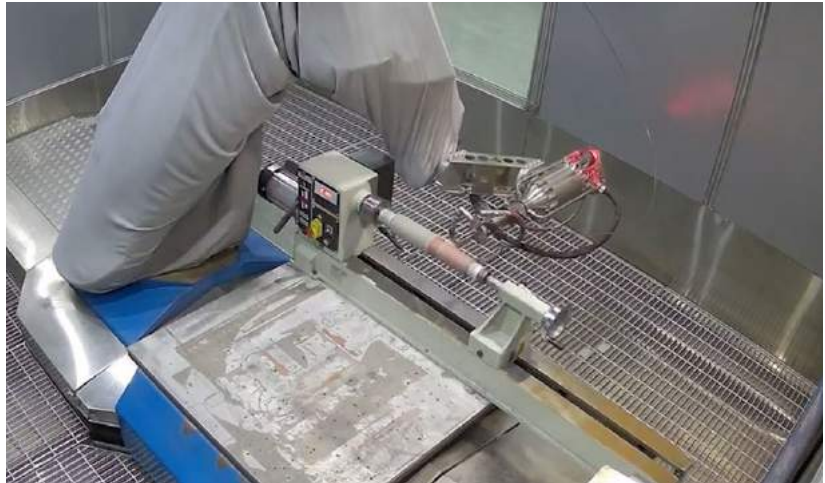
Cold spray can combine materials with vastly different melting and solidification ranges. Here, Titomic's TKF 1000 modular AM system is using Inconel 718, pure titanium and copper to create a hybrid part (Courtesy Titomic)
