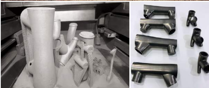
RAM3D has additively manufactured titanium parts for Sturdy Cycles bicycles, including its Road Race model (Courtesy RAM3D / Sturdy Cycles)
