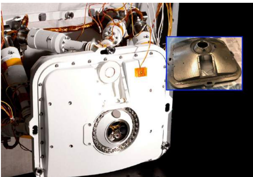
Five of the eleven metal AM parts are in Perseverance's Planetary Instrument for X-ray Lithochemistry (PIXL), shown here opening its dust cover during testing at NASA's Jet Propulsion Laboratory (Courtesy NASA/JPL-Caltech)
