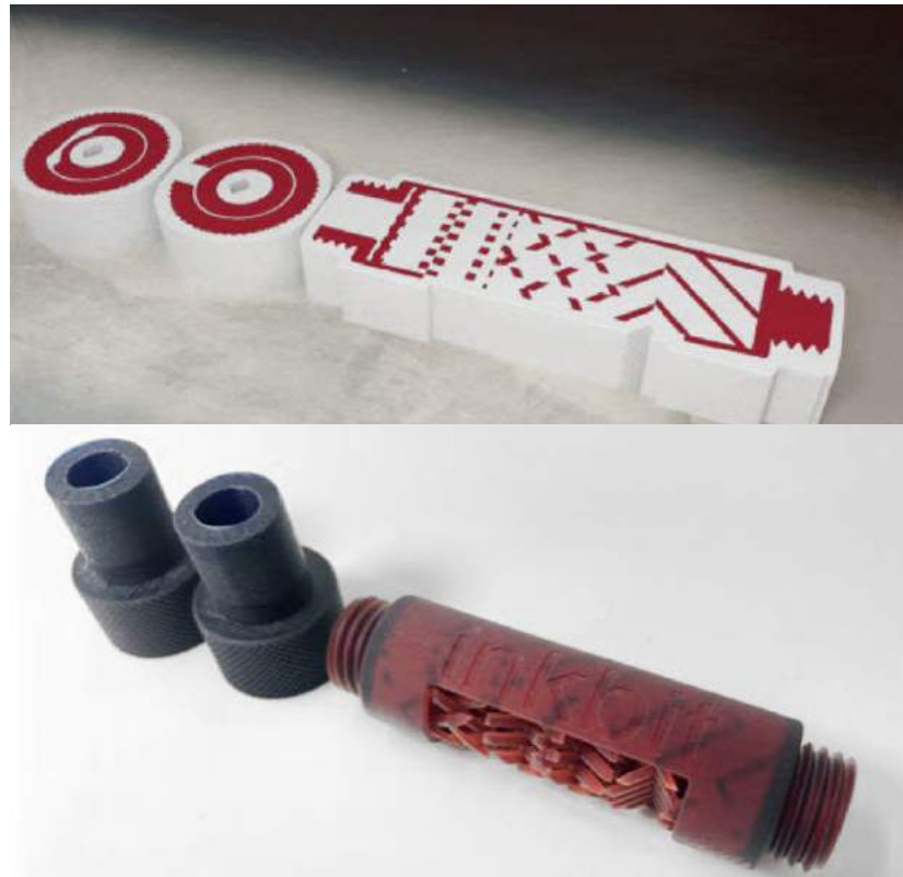
Fig. 3 The image on the top shows the scan of a measured layer, with support material (white) and the actual part (red), which trains the algorithm to make adjustments and improve. The final part is shown below (Courtesy Inkbit)
