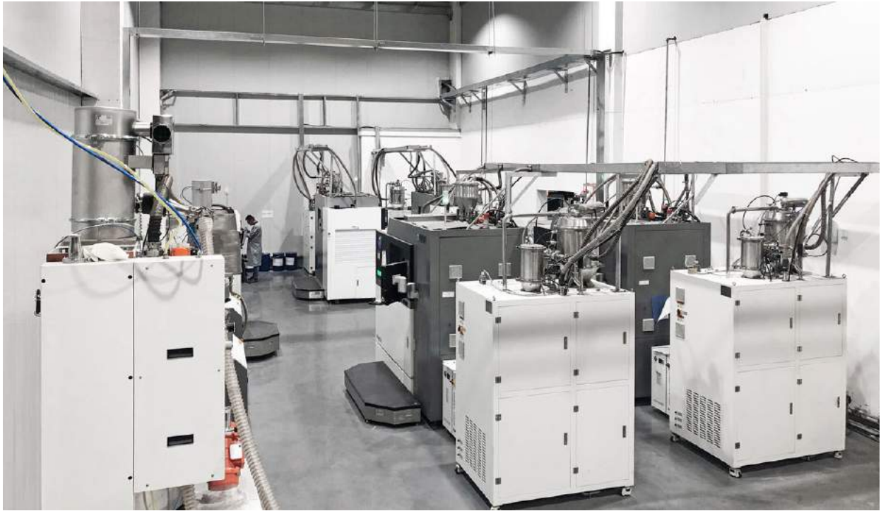
Fig. 6 Falcontech's AM production floor, with Farsoon metal AM machines, including FS421M, FS301M and FS271M (Courtesy Falcontech)
