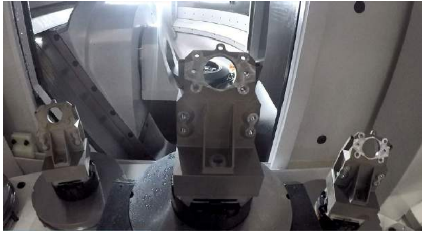
Fig. 6 BuildPal build plates benefit from the ability to use automated pallet handling for workflow optimisation (Courtesy System 3R)
