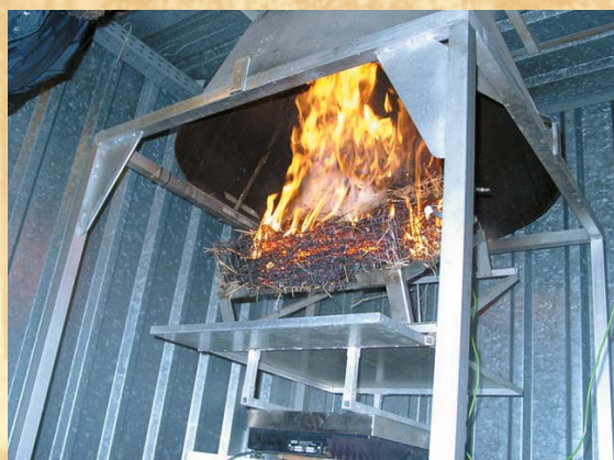
Laboratory fire for investigation of climate relevant properties of biomass burning aerosol.
