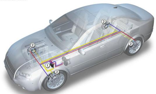
If the wheels lock when the brakes are fully applied, the ability to steer is lost and the vehicle can become uncontrollable. The task of the anti-lock brake system (ABS) is to permanently and effectively stop the wheels from locking, thereby stabilising braking. This is achieved by repeatedly and intelligently reducing and increasing the brake pressure, a procedure known as pressure modulation.
