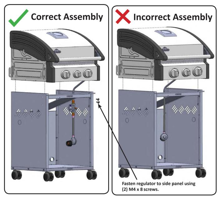
All cylinders 7kg or larger must be placed outside the enclosure (under the right side shelf) on level ground. The hose assembly must be routed through the knock out hole in the right side panel.
