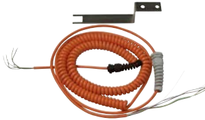
920081155550 Spiral cable 5 x 0,5 qmm, 0,8 m spiraled / 5m stretched.
