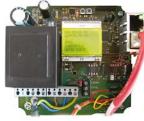
NDA008 Repeater module with integrated router.
