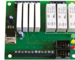
NDA030 K30 expansion module for D-Pro Automatic to add further inputs, outputs and to control traffic lights.
