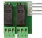
NDA040 For optional potential free outputs.
