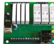
NDA030 For a two-way traffic light and extra programmable inputs/outputs
