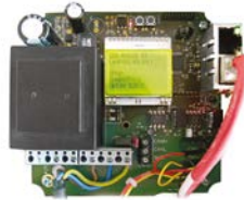
NDA008 K65 module for D-Pro Automatic control unit, for remote control (combined with NDA006 module).
