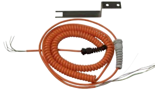
920081155516 Spiral cable 5 x 0,5 qmm, 0,8 m spiraled / 1,6 m stretched.
