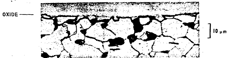
PLATE 3. Metallographic cross section of specimen shown in Plate 2 in region of maximum erosion corrosion loss.
