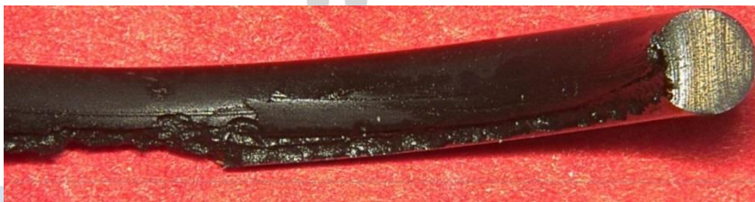
Fig. 17: Damage pattern air in hydraulic oil, the damage is found on the pressure side in contrast to gap extrusion.
