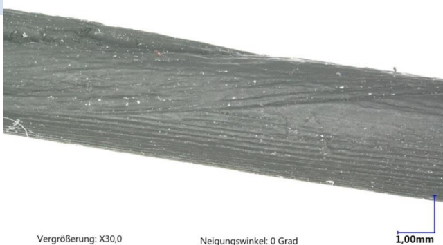
Fig. 11: Damage to an O-ring by a sharp-edged groove and dynamic pressure loads, this led to a twisting of the O-ring in itself
