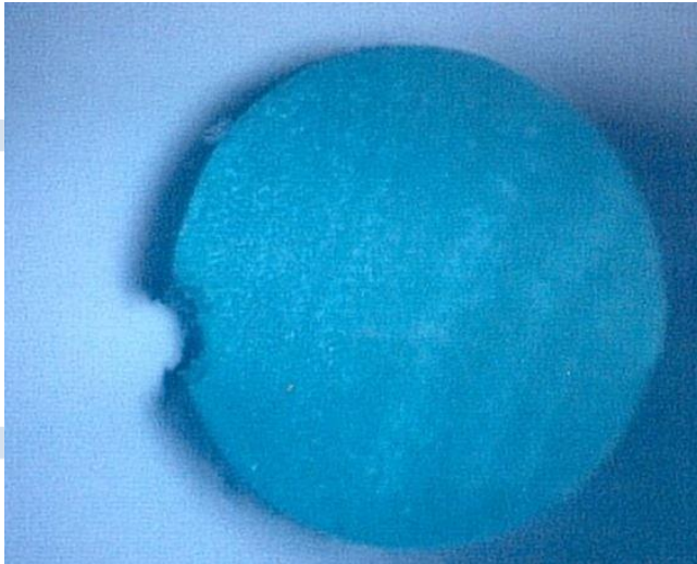
Fig. 7: Damage to an O-ring at the grooved phase due to high pressure rise rates
