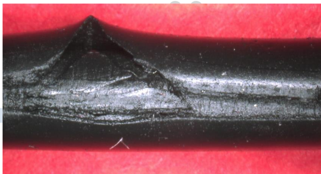
Fig. 10: Top view of an O-ring damaged by gap extrusion, section from Fig. 9
