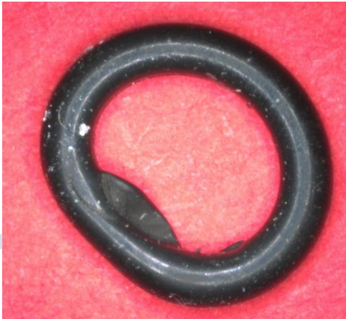
Fig. 16: Damage caused by a mounting error (compression)
