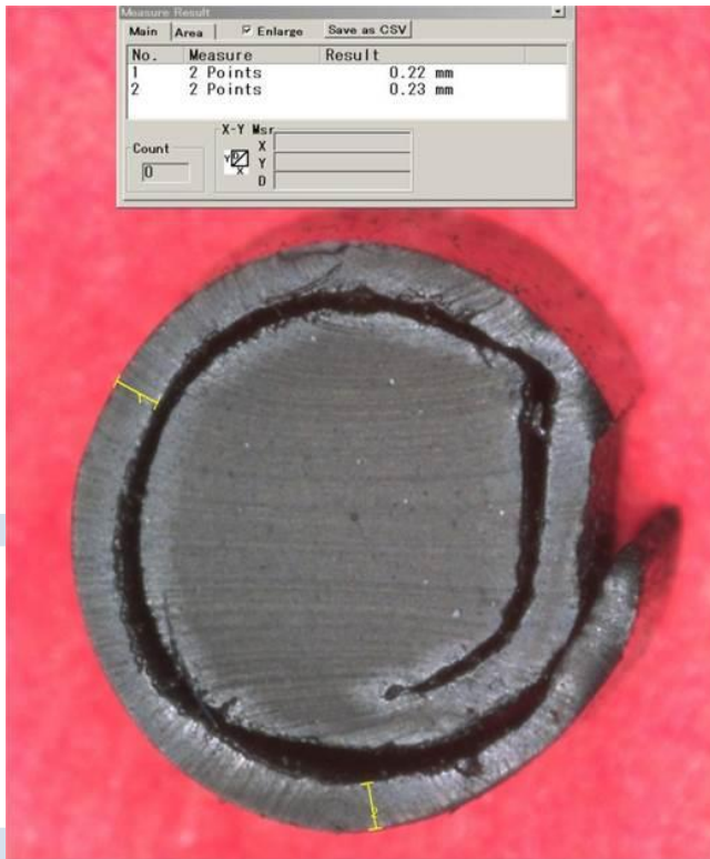
Fig. 9: O-ring damaged by gap extrusion (NBR 70 ShA at a gap of 0.2 mm and a pressure of 200 bar) in cross-section: atypically and strongly formed due to a sharp groove edge
