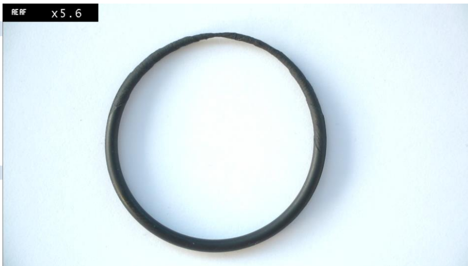
Fig. 8: O-ring after gap extrusion due to too large gap dimension: The area with the smallest remaining cord thickness (top of picture) represents the beginning of gap extrusion and is the point at the circumference with the largest gap dimension between piston and cylinder.
