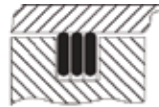
YH Series QH Series Internal - Light Duty 1 set = 3 individual rings (rings rotate with bore only)
