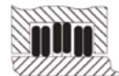
YSKD Series QSKD Series External - Heavy Duty 1 set = 3 individual rings (2 rings rotate with shaft & 1 ring rotates with bore)
