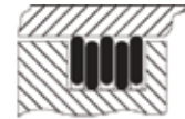
YHK Series QHK Series Internal - Medium Duty 1 set = 5 individual rings (3 rings rotate with bore & 2 rings rotate with shaft)
