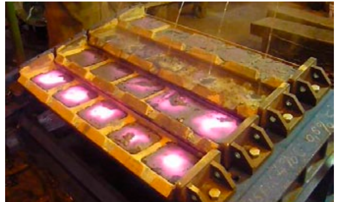
Shop testing - Water cooling after casting
