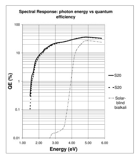
Figure (5) shows the spectral response of two S20 tubes and a solar blind tube plotted as quantum efficiency as a function of photon energy. The responses tend to peak at around 4.8eV.
