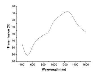
Figure (6) Transmission of S-1 photocathode as a function of wavelength
