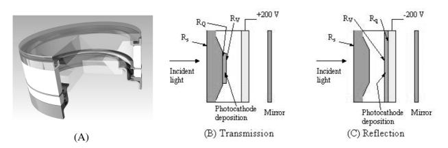
Figure 1: (A) Experimental test cell with photocathode window and rear window with ITO coating (or nickel mesh for UV cathodes) on inside surface for photo-electron collection. (B) Schematic test set up for transmission-mode testing showing the reflection interfaces, Rs, RQ, and RV. (C) Same as B, but for reflection measurements. The 200 V bias to ground is used to measure the photocurrent signals, S.
