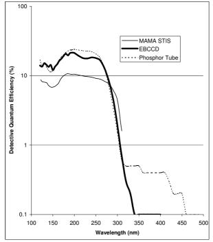
Figure (3) Comparison of detective quantum efficiency of the Photek EBCCD tube built for Rutgers University with the STIS MAMA detector. A variant of the Photek tube using a phosphor screen instead of an EBCCD is also shown.
