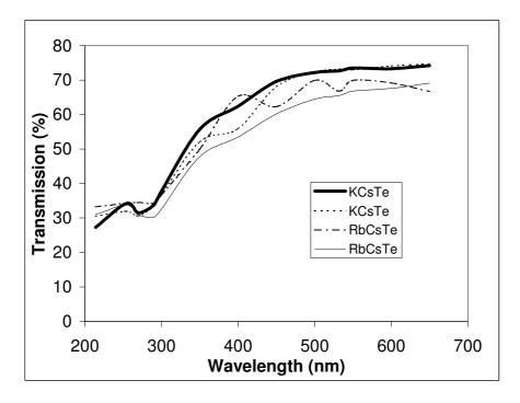
Figure (4) Transmission results as a function of wavelength for telluride photocathodes on a test cell with a sapphire rear window. The entrance window was  $MgF_2$ . Tubes 13050823 and 13060223 were RbCsTe, the other two were KCsTe.
