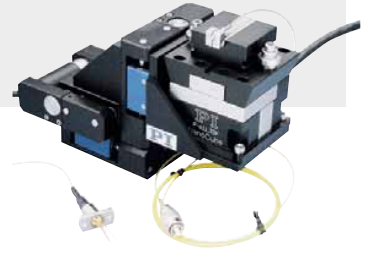
F-130 fiber alignment system consisting of an M-110 XYZ positioning system and a P-611 XYZ Piezo-Nano Positioning system. This combination can be operated by the C-880 controller or NI controllers (request our technote!)
