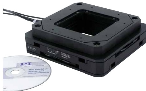
M-686 open-frame stage with P-541.2DD piezo scanner on top, providing a resolution of 0.1 nm and a scanning range of 30 x 30 \mu\text{m} . The system height of the combination with the P-541 XY (or Z) piezo scanner is only 48 mm
