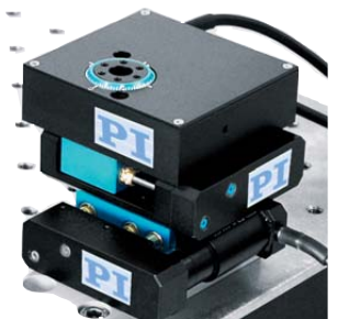
XY \theta_z micropositioning combination consisting of (from top to bottom) M-116 micro rotary stage and two M-111 translation stages (M-110.01 adapter for mounting the M-111 on a honeycomb breadboard)
