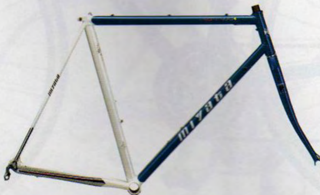
Team Miyata • STB Chrome-Moly Frame • Oversized Top Tube • Aluminum APA Bonded Fork
