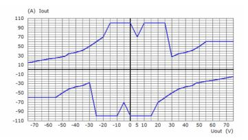
Continuous Output Current vs. Output Voltage (THD + N < 1%) Uout= +/- 27V Supply Voltage: Auto Blue: AC Limit Red: DC Limit
