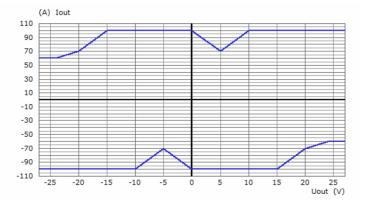
Short-Time Output Current vs. Output Voltage (THD + N < 1%) Uout= +/- 75V Supply Voltage: Auto Blue: Pulse Current Limit; 200ms Pulse, duty cycle=5 %
