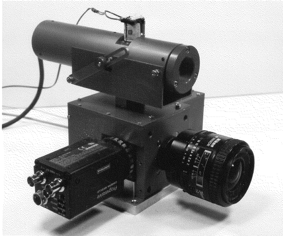
Figure 8.11 For 3D measurements, the shearography head is combined with all three illumination modules.
