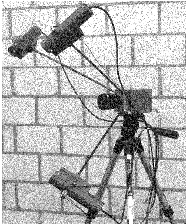
Figure 8.11 For 3D measurements, the shearography head is combined with all three illumination modules.
