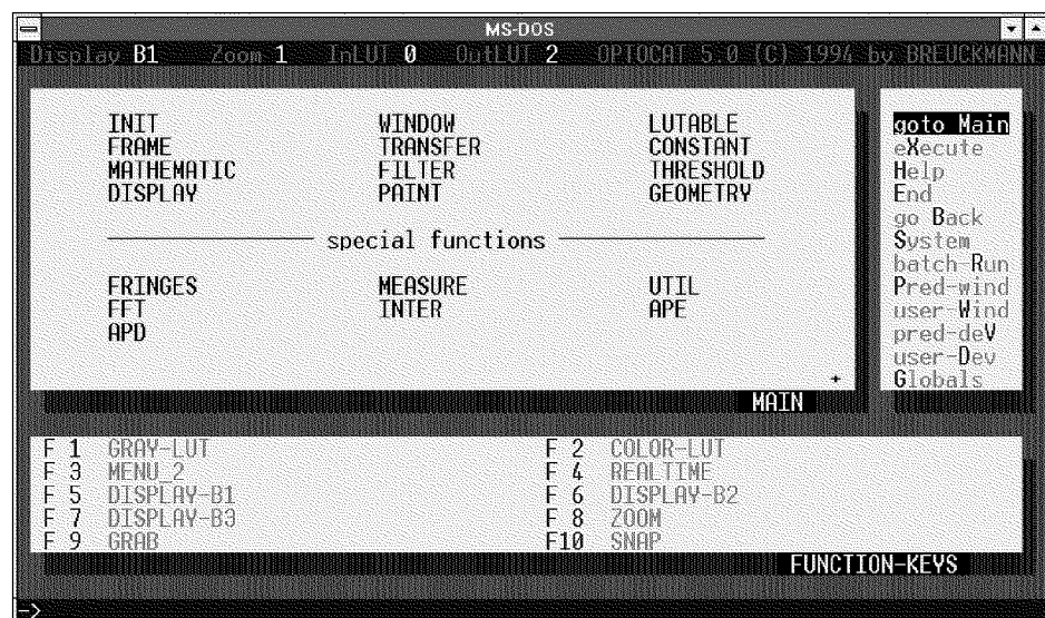
Figure 8.2 Main screen of the OPTOCAT program. In the upper left part, the command groups are shown, on the right side, special commands with their shortcuts are displayed and in the lower part the function keys. The last line on the screen is the command line. A second monitor is used to display the images.
