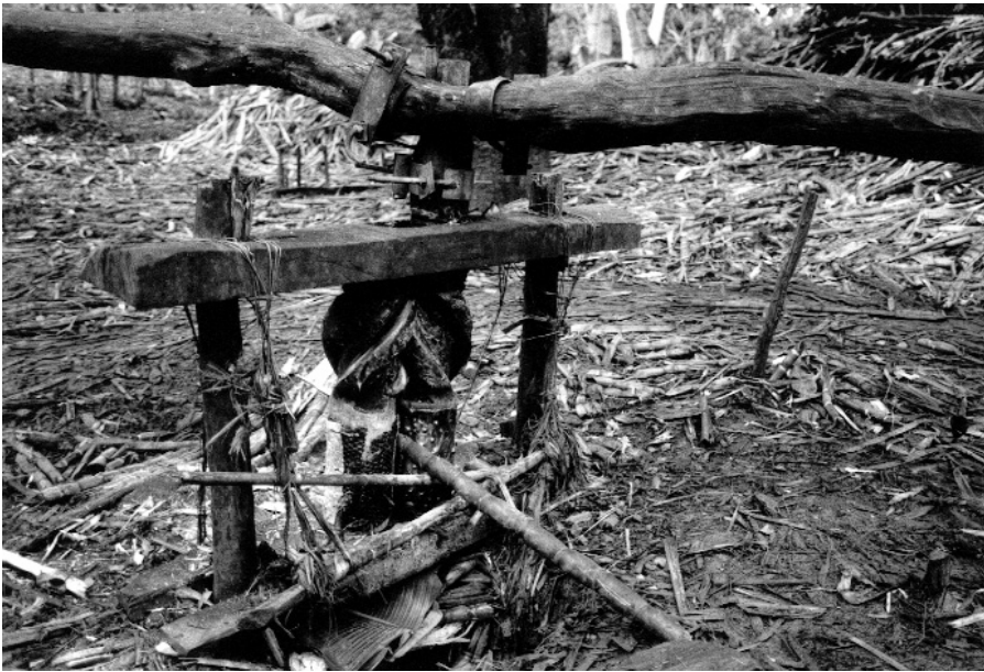
Fig. 3.7. The gears and handle of this sugarcane press in the East Usambara Mountains are constructed from native trees
