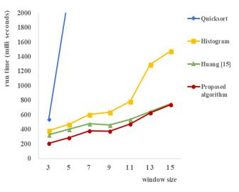
Figure. 6. Timing of median filtering algorithms and the proposed algorithm.
