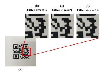
**Figure. 5**. Effect of median filtering. (a) Original RGB image, (b) The part of the image after applying the  $3\times3$  median filtering (c) The part of the image after applying the  $9\times9$  median filtering (d) The part of the image after applying the  $15\times15$  median filtering.
