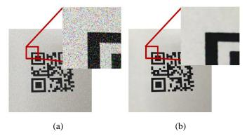
**Figure. 1.** Effect of median filtering. (a) Image before filtering, (b) Image after 3×3 median filtering.
