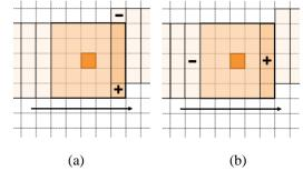
**Figure. 3.** Histograms update of the constant algorithm. (a) Update processing of the column histogram  $h_j$ . (b) Update processing of the kernel histogram *H*.
