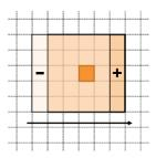
**Figure. 2.** Histogram update in Huang's algorithm (In this figure, n=5)
