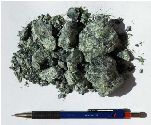
Fig. 14 Piece of sheared ophiolite, which has been disintegrated into flakes of weak serpentinite
