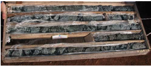
Fig. 13 Poor quality sheared serpentinite from the mountain of Orthrys in central Greece. Completely disintegrated peridotite with loss of blockiness and presence of clayey sections. Tunnel stability will be controlled by stress dependent rock mass failure with significant squeezing at depth. Depth of samples in photograph about 175 m, GSI 15–20
