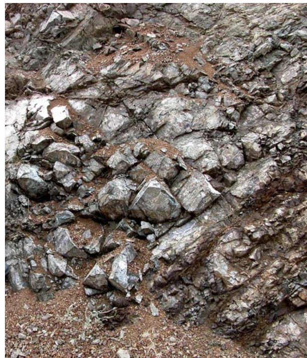
Fig. 9 Good quality surface outcrop of blocky structure in peridotite with fair (smooth, moderately weathered and altered) surface conditions of discontinuities. Width of photograph about 1.5 m. GSI~55
