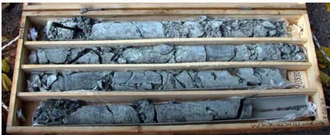
Fig. 11 Fair quality peridotite, from the mountain of Orthrys in central Greece, with discontinuities of low frictional properties due to the presence of films of serpentinised material. Blocky-jointed with short lengths of disintegrated or serpentinised sections. Tunnel stability will be controlled by structural stability of small blocks or by mild overstraining. Depth of the cores in photograph about 200 m. GSI 35 \pm 5
