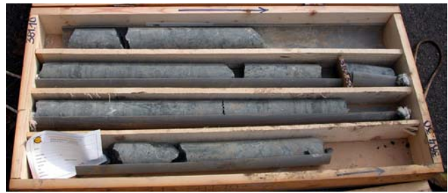
Fig. 8 Good quality peridotite from the mountain of Orthrys in central Greece. The conditions of the widely spaced discontinuities are only mildly affected by serpentinisation. Tunnel stability is controlled by occasional structural failures. Depth of the cores in the photograph about 380 m. GSI 80 \pm 5
