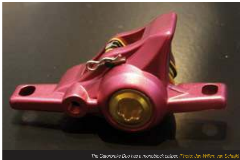
The Gatorbrake Duo has a monoblock caliper. (Photo: Jan-Willem van Schaijk)
