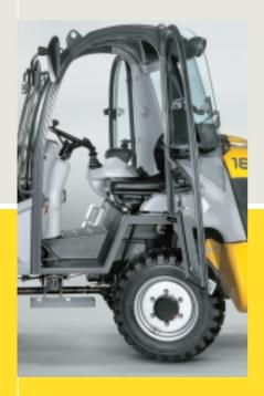
The 45% self-locking differentials in both axles tackle difficult terrain with ease, while the hydrostatic drive also provides effective braking.
