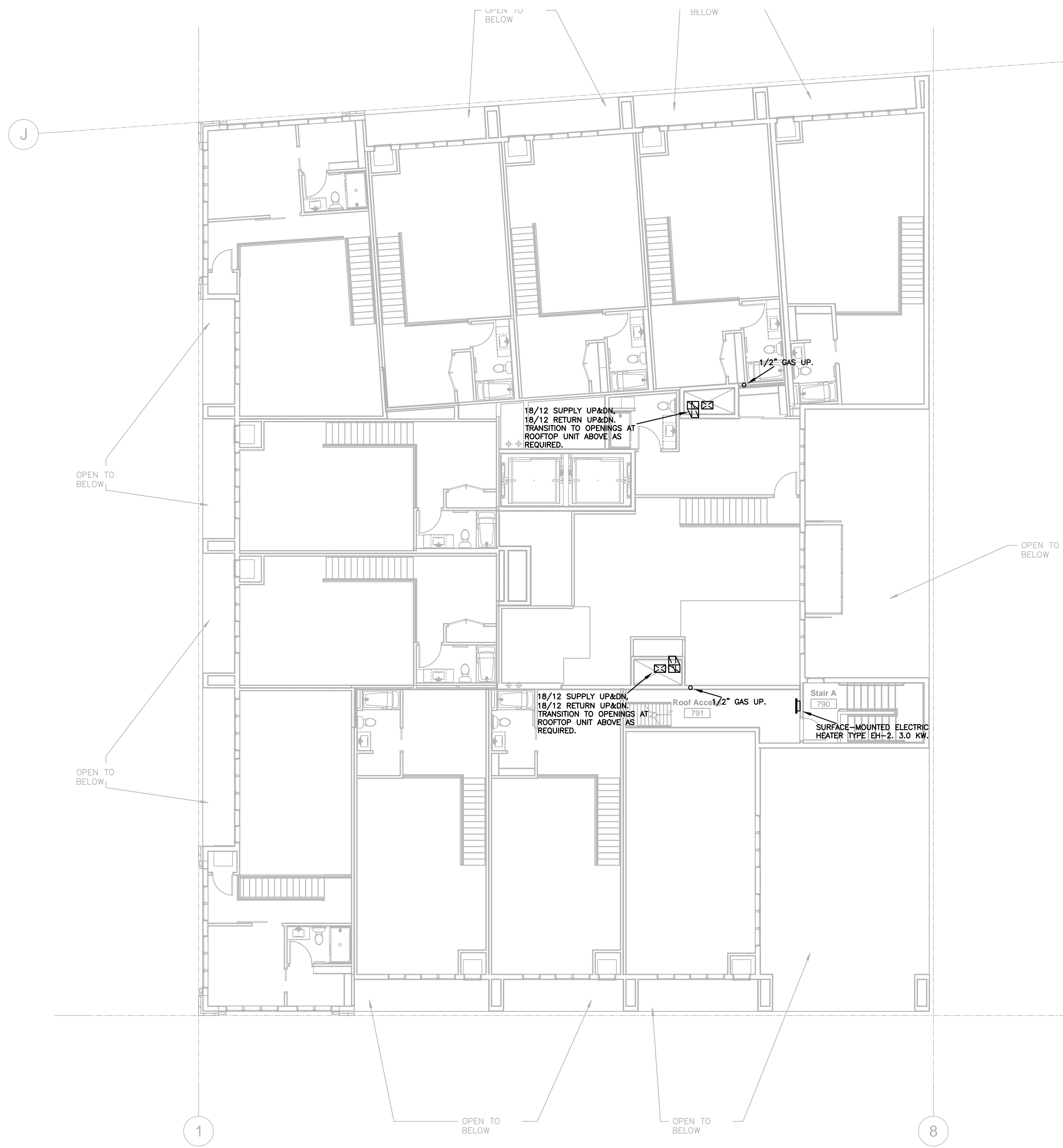
1 MECHANICAL PLAN - LEVEL 6 MEZZANINE 1/8"=1'-0"
