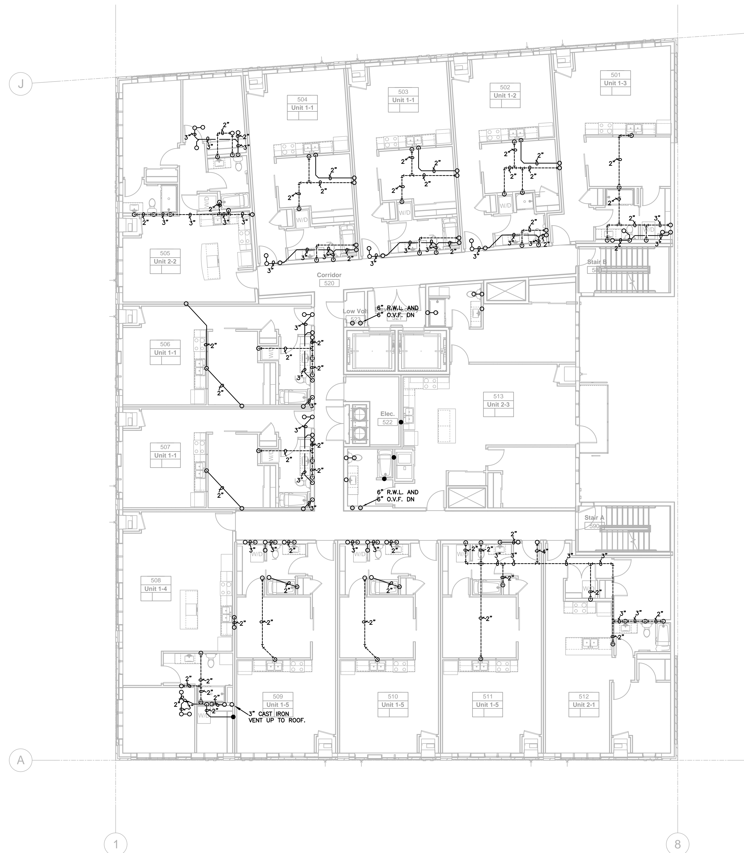
1 P350 DRAIN, WASTE, & VENT PLAN - LEVEL 5 1/8"=1'-0"
